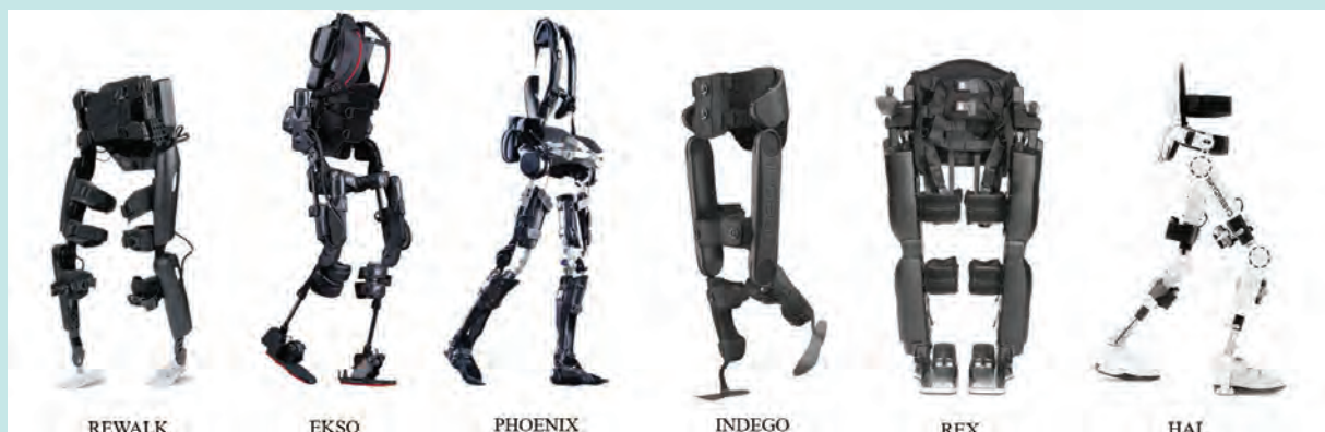
Figure 1. Commercially available lower extremity exoskeletons for locomotion assistance and/or rehabilitation of paraplegic patients
