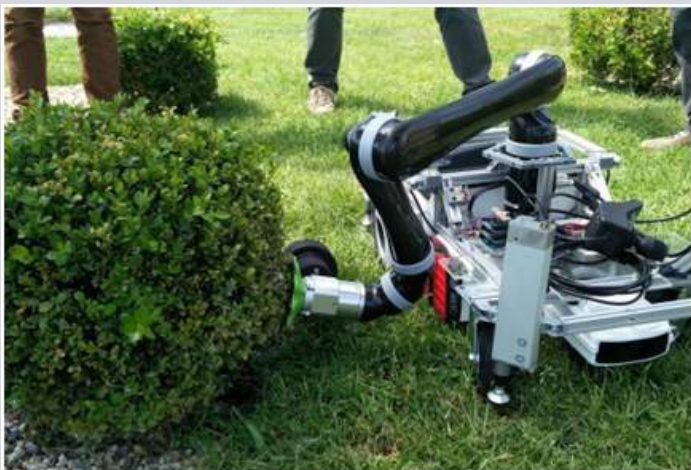
Figure 2 : “Trimbot” robot to trim bushes and prune roses
