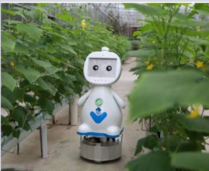
Figure 1 : AI powered and 5G enabled robot that monitors conditions inside a greenhouse
